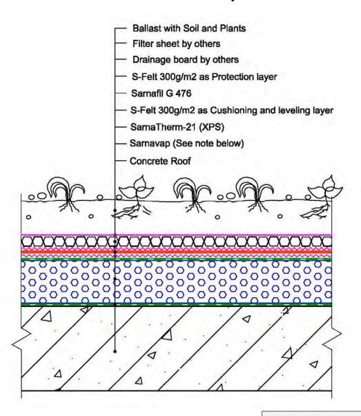
Positioning of Sarnavap to be according to local climate conditions.
