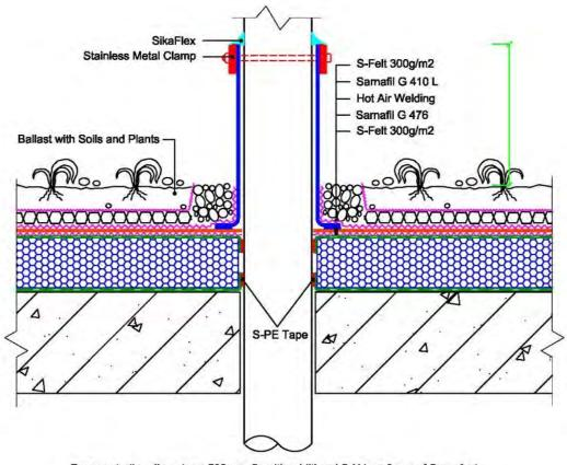
For penetration diameter > 500mm, fix with additional S-U bar, 3 pcs of Samafast SBF 6.0, S-PVC Welding Cord and S 327/ G410 L Cover strips.
