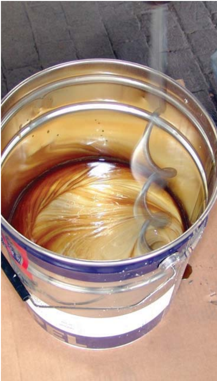
Picture 7: Mixing of SikaGlaze GG-735
