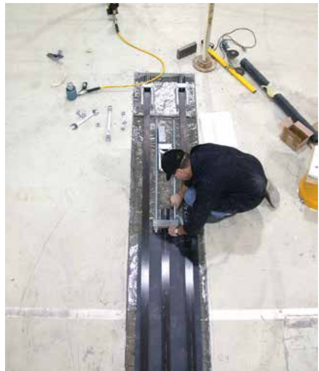
Plate and end-anchorage
