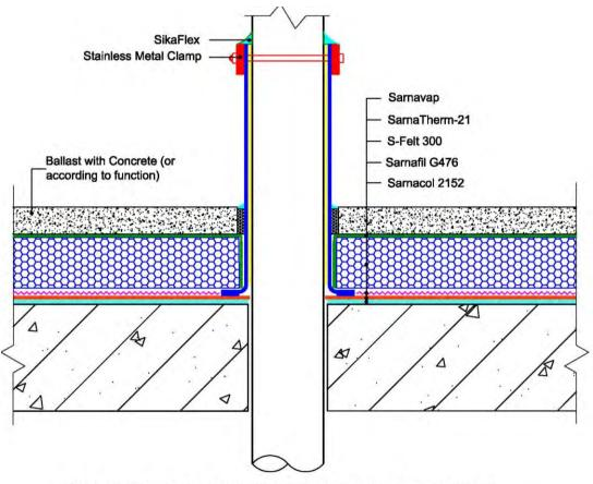
For penetration diameter > 500mm, fix with additional S-U bar, 3 pcs of Sarnafast, S-PVC Welding Cord and G410L Cover strips.
