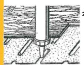
Apply the adhesive with manual or air-pressure gun into all cut-outs using the supplied triangular nozzle (width 8mm, height 10mm). All cut-outs must be filled.
