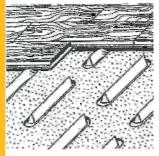
Position wood boards and firmly press the boards into the adhesive until they lay tight on the SikaLayer-05 mat. The wood boards can then be joined together using a hammer and an impact block.
