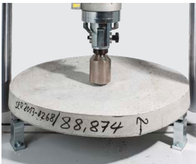
Round panel test: ASTM C1550
