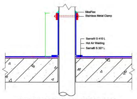
For penetration diameter > 500mm, fix with additional S-U bar, 3 pcs of Sarnafast SBF 6.0, S-PVC Welding Cord and S 327/ G410 L Cover strips.
