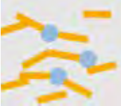
Moisture in concrete and a well distributed dosing of PP micro-fibre
