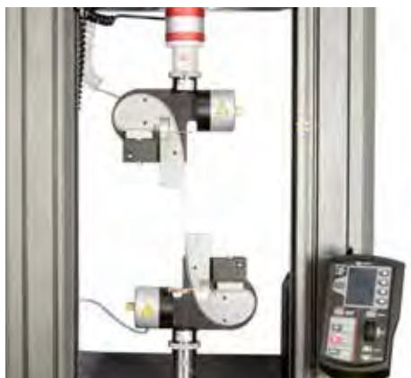
Figure 4.4.1.2: Snubbing clamp referred to ASTM D 2256-02
