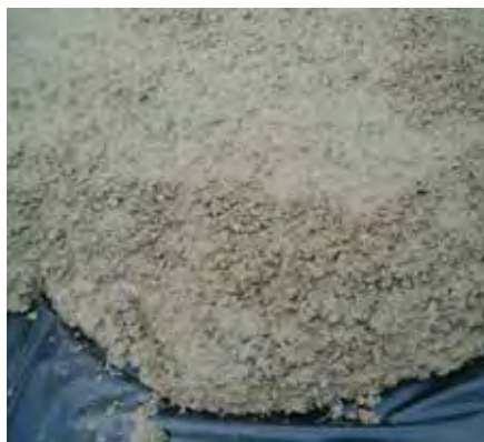
Figure 4.1.1: Fresh concrete without balling
