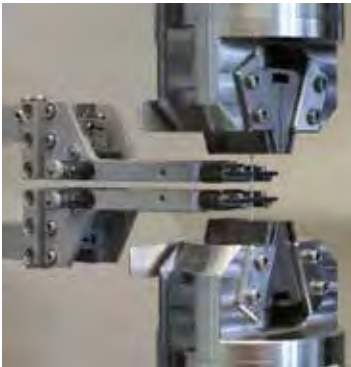
Figure 4.4.1.1: Universal Testing Machine with a flat-faced clamping system, incorporating a tactile extensometer for very precise determination of the strain
