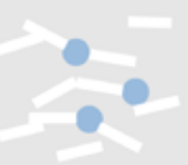
When the rising heat source reaches a temperature of 160°C (360 degree F), the PP micro-fibres melt.
