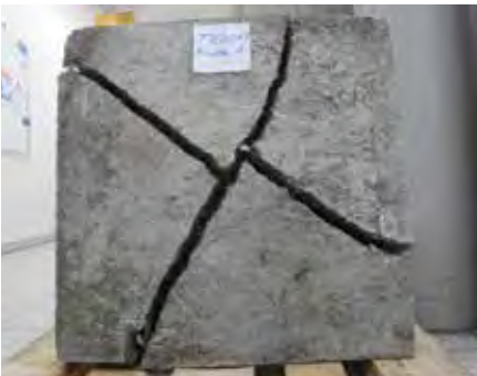
Figure 8.2.1.2: Underside view of tested square panels
