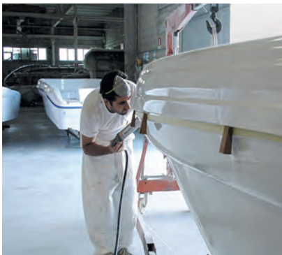
Fig. 8 Sealing with Sikaflex®-295 UV
