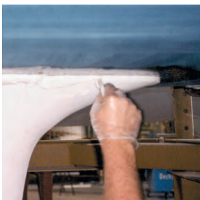
Fig. 13 The joint is tooled off and finished
