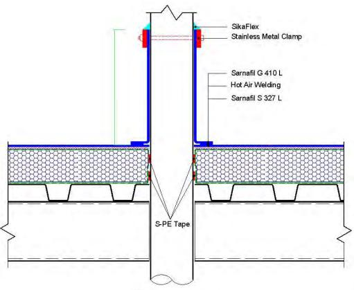
For penetration diameter > 500mm, fix with additional S-U bar, 3 pcs of Sarnafast SBF 6.0, S-PVC Welding Cord and S 327/ G410 L Cover strips.
