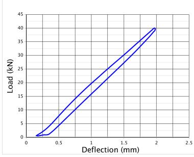
Static stiffness determined analogous to DIN 45673-1. Test specimen dimensions  $1000 \times 180 \times 25$  mm.
