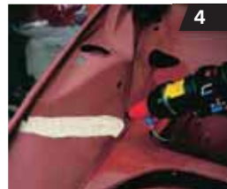
Narrow angle spray application for sealing flush seams.
