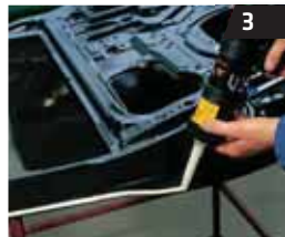
Bead application to seal lock seams, e.g. on door assembly or in engine compartment.
