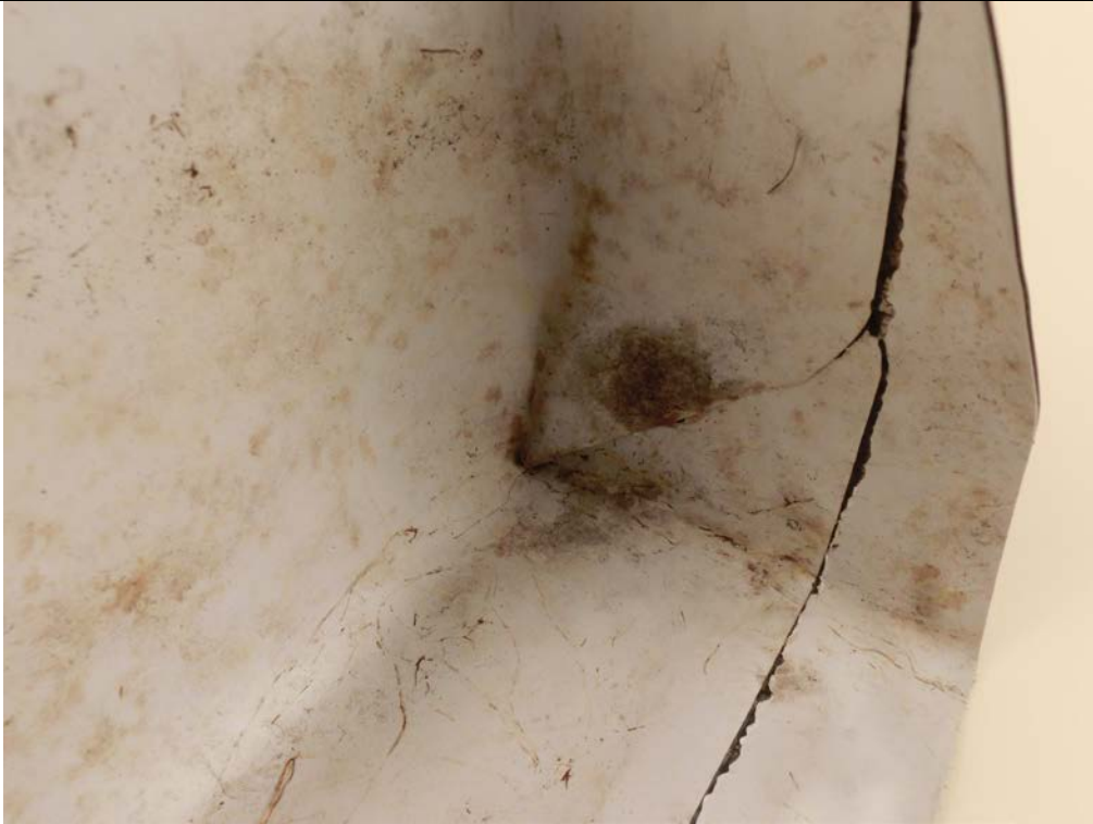
Figure 3: Membrane surface with wall corner made by a double counterlaid fold
