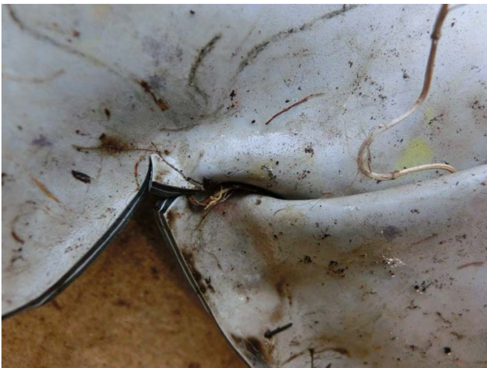
Figure 4: Corner made by a double counterlaid fold with rhizome penetration
