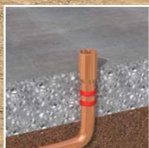
Sealing of penetrations
