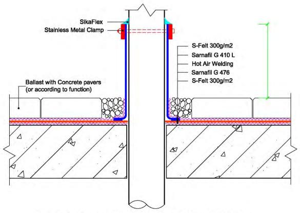
For penetration diameter > 500mm, fix with additional S-U bar, 3 pcs of Sarnafast SBF 6.0, S-PVC Welding Cord and S 327/ G410 L Cover strips.
