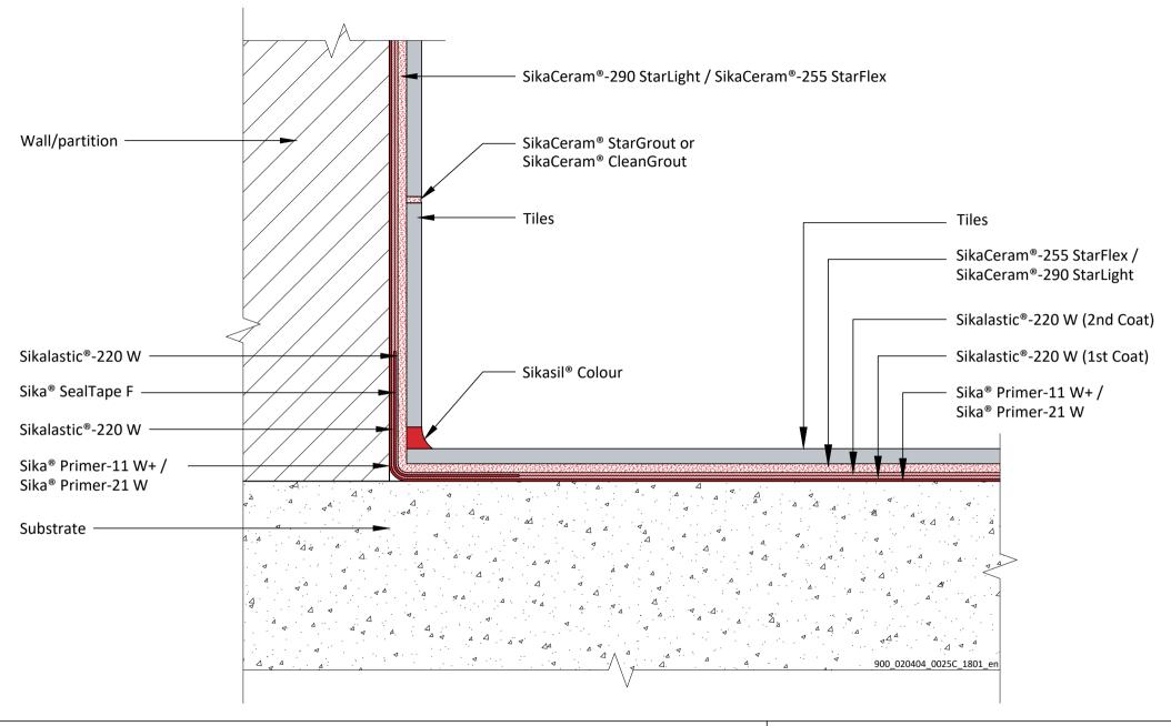
**DETAIL FOR BUILDING FINISHING, TILE SETTING** Waterproofing and tiling according ETAG022 900\_020404\_0025C\_1801\_en June 2021 Sika (NZ) Ltd
