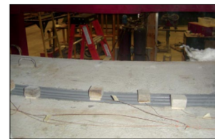
Thermocouples register no more than 248°F (120°C)
