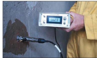
Permeability Testing of Concrete
