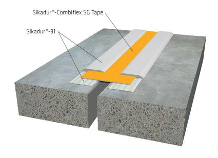
**Flexible polyolefin tapes:** Sikadur Combiflex® SG-10 P, Sikadur Combiflex® SG-20 P
