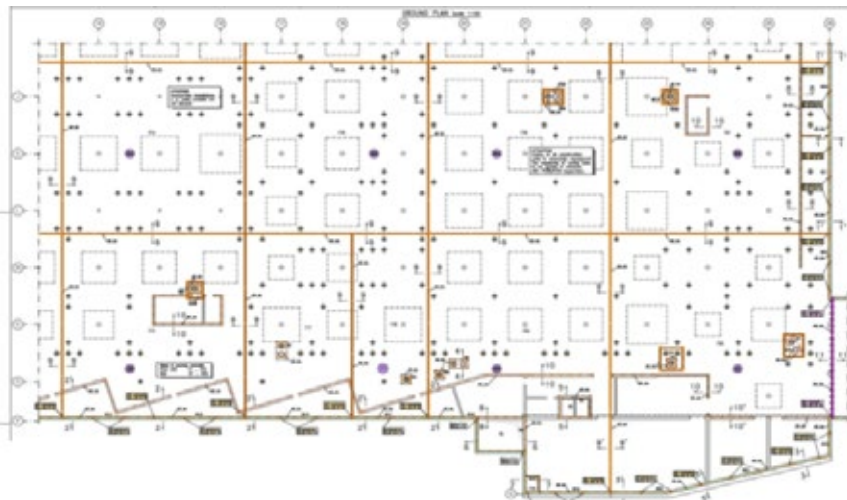
Figure 9.3: Optimized definition of joint layout on a base slab to reduce cracks.
