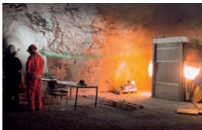
Fig. 8.5.1: In special furnace chambers fire trajectories can be replicated, panels tested and subsequently evaluated. Temperature development is measured and recorded at various depths.
