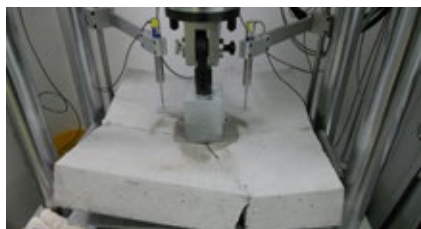
Fig. 8.11.3: Special testing for sprayed concrete: Energy absorption testing of fiber reinforced sprayed concrete to EN 14488-5.
