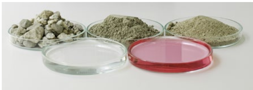
Fig. 4.2.2: Mix design ingredients of concrete: Gravel, water, cement, superplasticizer, sand (from left to right)
