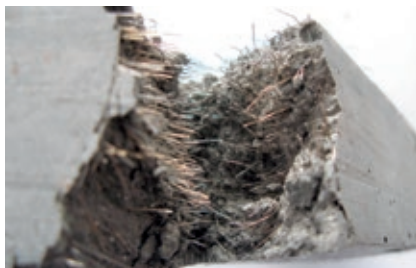
Fig. 8.9.1: High strength and above all ultra high performance concrete (UHPC) are usually fiber-reinforced. Depending on the requirements, synthetic and/or steel fibers are thereby employed in large quantity.
