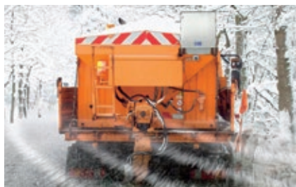
Fig. 8.3.3: Scattered de-icing agent considerably intensifies the reaction upon freezing of water and leads to substantially greater damage in areas of concrete close to the surface.
