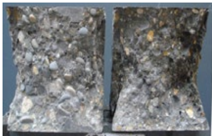
Fig. 8.9.2: The differences in the quality of aggregates and the w/c-ratio used determines whether fractures occur in the aggregates or the cementitious paste at the point of maximum loading. The picture shows a reduction of the w/c-ratio from 0.32 (left) down to 0.28 (right).
