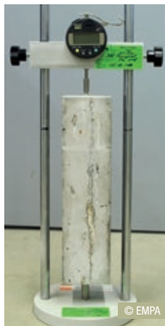
Fig. 8.6.2: The increase in volume due to the strain resulting from ASR becomes perceptible by measurement of a change in length of test specimens. Ordinarily the specimens are stored under intensified conditions (temperature, humidity, applied load) in order to accelerate the reaction.
