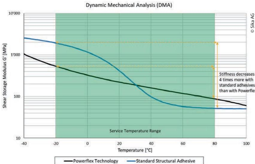
**Figure 1** > Comparison of DMA between "Powerflex" technology and standard structural adhesive in commercial transportation
