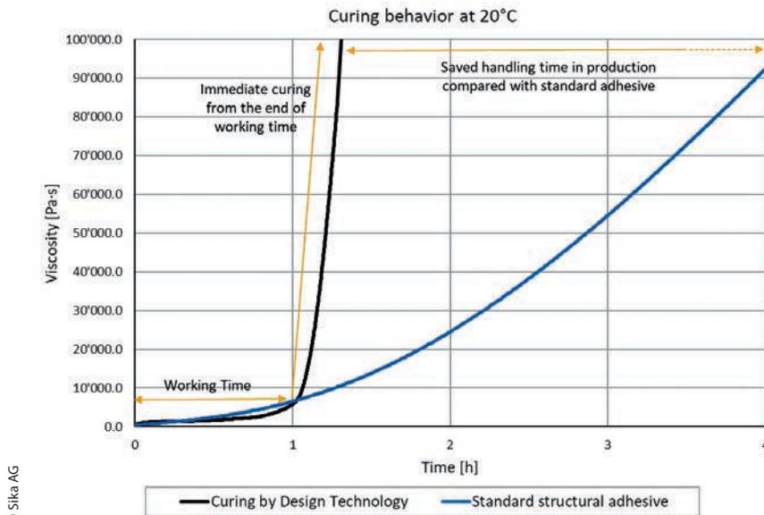
**Figure 4** > Comparison of curing behavior between 'Curing by Design' technology and a standard structural adhesive with same working time
