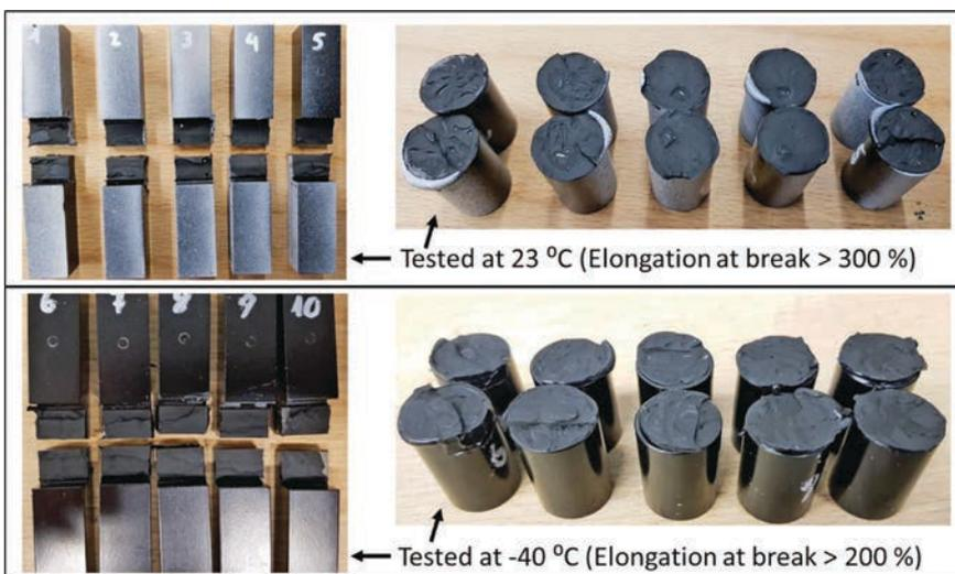
**Figure 2** > Cohesive failures of 'Powerflex' adhesive on e-coated steel in 'Thick Adherent Shear Tests' (TAST) and butt joint tensile tests at  $23\text{ }^\circ\text{C}$  and  $-40\text{ }^\circ\text{C}$
