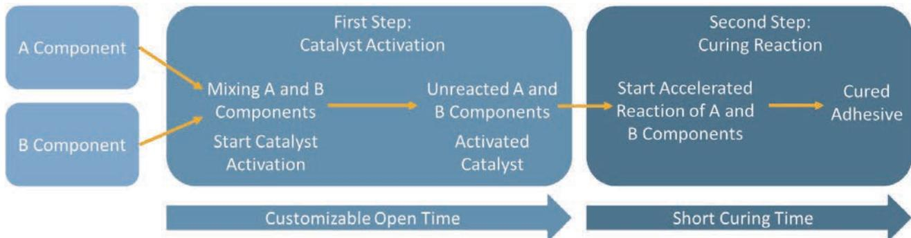
**Figure 5** > 'Curing by Design' working mechanism (schematically)
