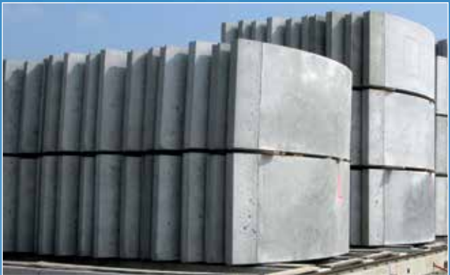
Segment production Weinberg Tunnel, Switzerland
