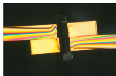
Fig. 4 Screwed sample. The force line indicate a direct transmission of the forces from one part of the sample through the screw to the other part of the sample
