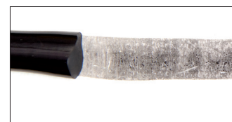
Pic 5: Bad adhesion. Nothing or a thin film remaining on the substrate
