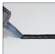
Pic 1: Apply bead on original substrate
