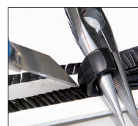
Pic 2: Peel of the aged bead using a plier
