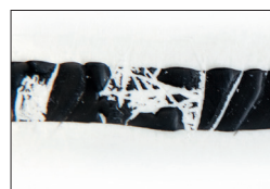
Pic 4: Good adhesion with some cohesive failures in the substrate
