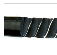
Pic 3: Sample with an excellent adhesion
