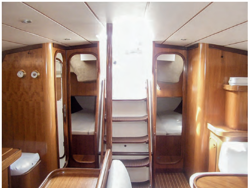
Fig. 13 High-quality lightweight panels finished in traditional high-gloss wood veneer and bonded using Sikaflex®-252
