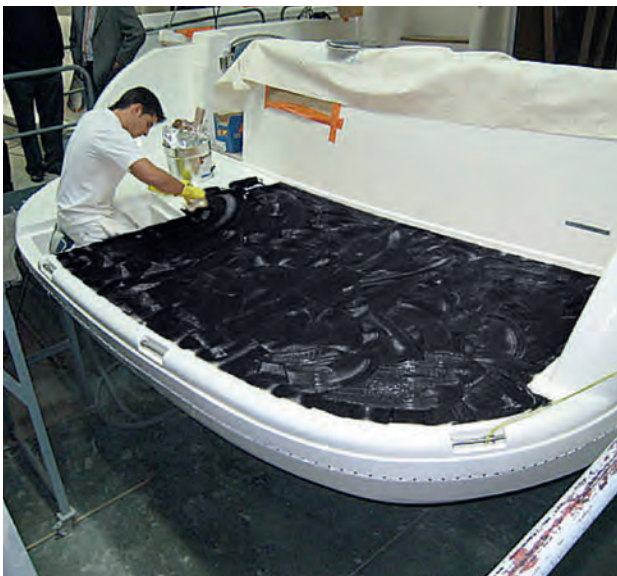
Fig. 26 Application of Sikaflex®-298
