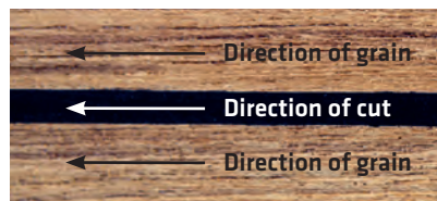
Fig. 33 Always ensure that the direction of cut is with the grain to avoid 'digging-in' damage to the sides of the planks
