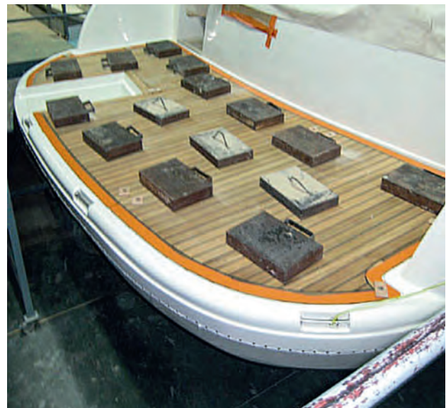
Fig. 27 Holding in place with weights
