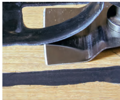
Fig. 49 Picture Removal overstanding Sikaflex®-290 DC PRO with a vibrating scraper power tool
