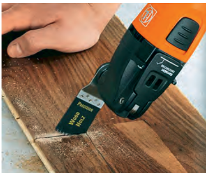
Fig. 48 Cutting planks with vibrating knife
