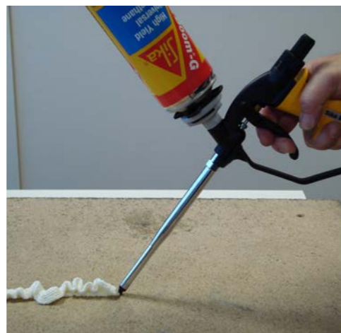
A tighter trigger squeeze = a wider bead of foam
