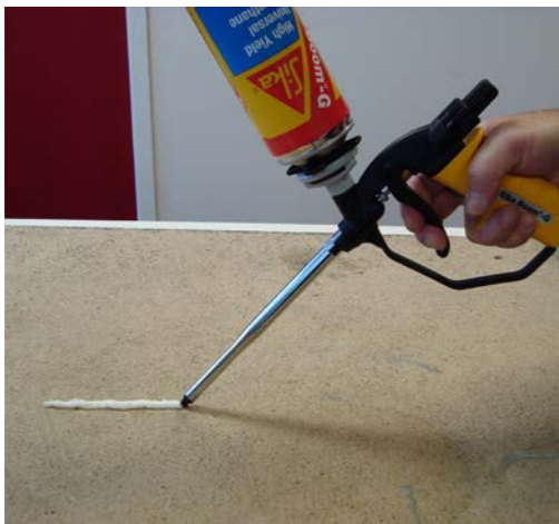
A light trigger squeeze = a fine bead of foam
