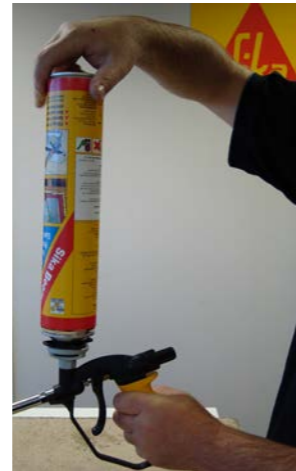
With the can facing away from your body, screw the can onto the Sika Boom-G Gun. Make sure the can is "hand tight". You may hear a hiss as the can attaches to the adaptor.
